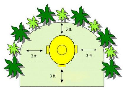
A <u>3-foot clear space</u> shall be maintained around the circumference of fire hydrants... unobstructed access to fire hydrants shall be maintained at all times.
